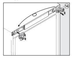
■ Unscrew bearing block <sup>1</sup>, turn it around and fit it on the opposite side.
